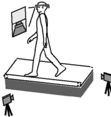
Figure 17: Computer managed obstacle avoidance on a treadmill [2]
