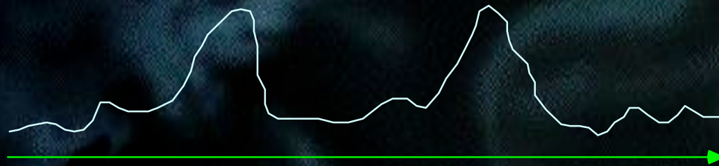
continuous electrical signal from one scanline
