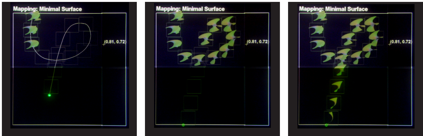
Figure 4: The Geometer's Workbench interface is designed to compensate for the latency of mathematical computations, by queuing calls to Mathematica and displaying results as they become available rather than blocking. Here we show the evolution of the display as the user draws on the Multipoint area. Notice that the pen trail is resampled by the system and that the trail of samples is updated progressively as the results of mathematical computations become available.
